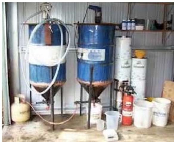
In this photo I had begun to store the 5 gallon pails in 55 gallon drums that made it easier to manage. I put a tap on the bottom so the potential bio diesel could be easily taken out.
